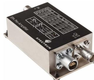
For the acquisition of extremely small voltage levels with a high bandwidth a series of external amplifiers is available. Each of the one channel amplifiers is working with a fixed input impedance and allows - depending on the bandwidth - to select different amplification levels between  $\times 10$  (20 dB) up to  $\times 1000$  (60 dB). Using the external amplifiers of the SPA series voltage levels in the  $\mu\text{V}$  and  $\text{mV}$  area can be acquired.
