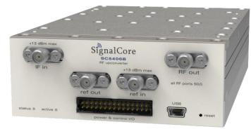
The output compression-to-noise dynamic range is typically 150 dB and the spurious-free dynamic range is better than 110 dB. As an example, for a 0 dBm output signal the SNR is better than 130 dBc while achieving -70 dBc 3<sup>rd</sup> order inter-modulation distortion (IMD3). The SC5406B also has a wide gain range. Output signal levels as low as -110 dBm and as high as +16 dBm can be achieved.
